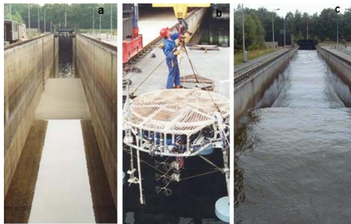
Figure 6. (a) Photograph of the flume used to collect the measurements. (b) The instrumented tripod platform, STABLE II, used to make the acoustic measurements. (c) A wave propagating down the flume.
