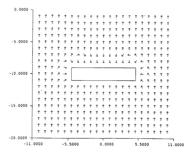
Figure 1: The direction of the Kelvin impulse for a bubble at different locations relative to a rigid cylinder.
