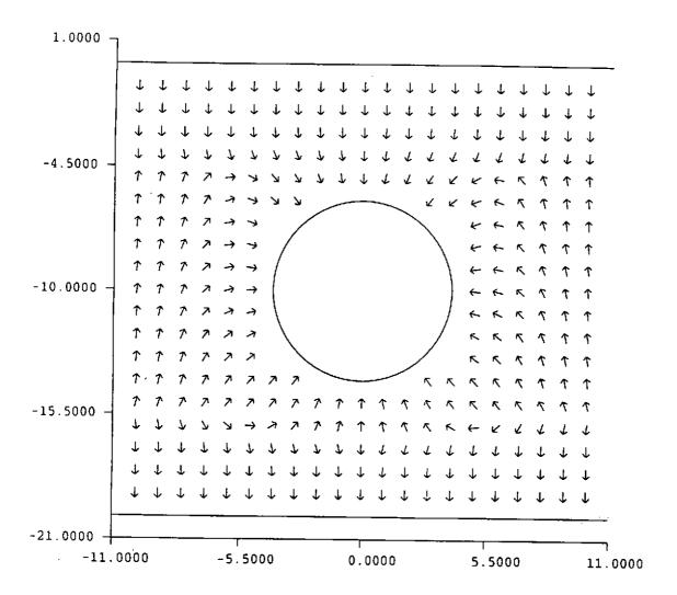
Figure 2: The direction of the Kelvin impulse for a bubble at different locations relative to a rigid sphere in shallow water.
