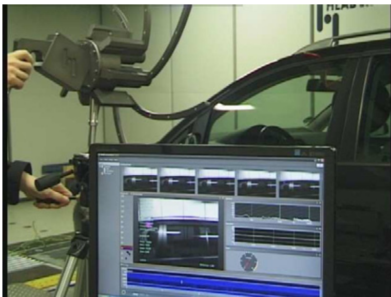
Figure 8: Online evaluation. The software (foreground) displays online the current source map while the array is moved around the vehicle.
