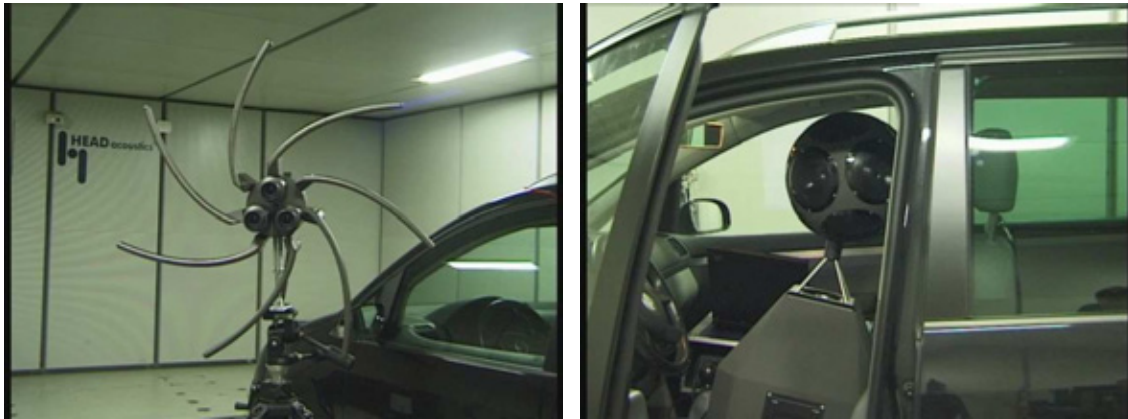
Figure 7: Leakage detection with microphone array (left picture) and point source inside the vehicle (right picture)
