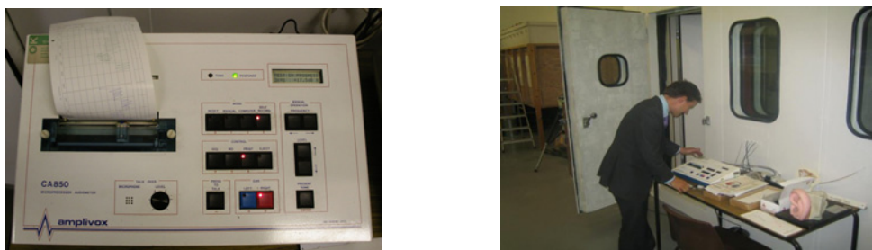
Figure 4. Environmental chamber with double layer doors and Amplivox audiometric equipment.
