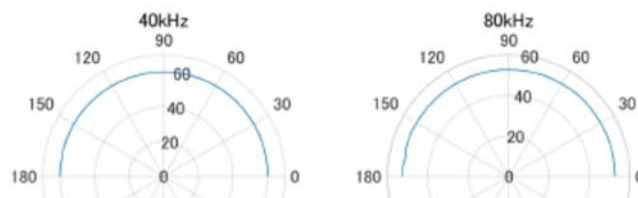
Fig. 6 Directional pattern of LIB measured in an anechoic chamber. The peak values are plotted.
