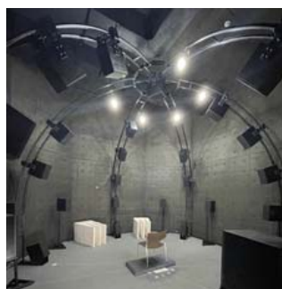
Fig. 15 Semi-anechoic chamber for presentation.
