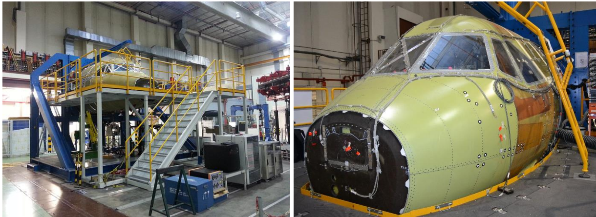
Figure 1: Clean Sky / Green Regional Aircraft MT2 cockpit demonstrator and test rig developed by Airbus Defence and Space.
