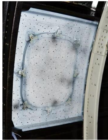
Figure 7: Speckle pattern painted on the passenger window (interior view)
