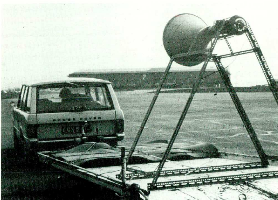
Figure 3 Measuring effect of turbulence at target vehicle
