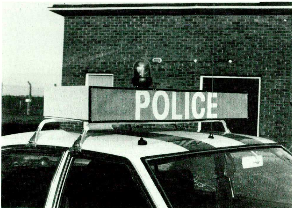
Figure 4 Prototype loudspeaker array in cowling
