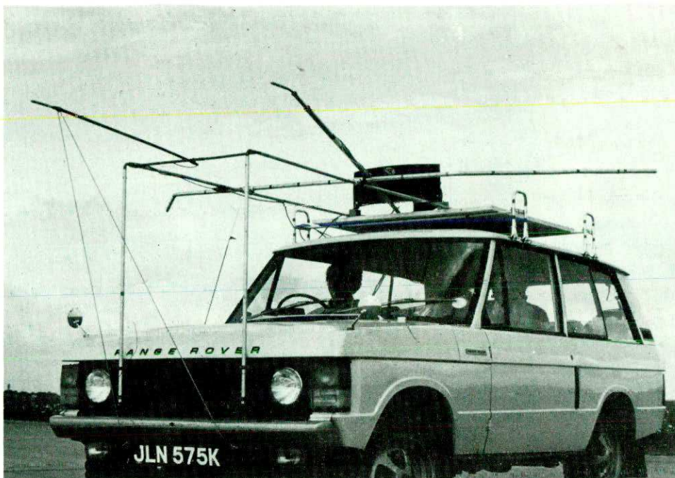
Figure 2 Measuring effect of turbulence on sound source
