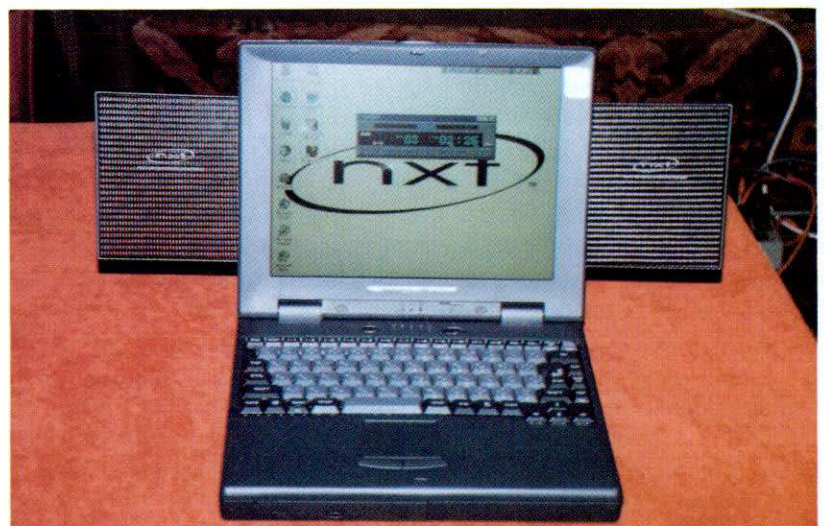
Photo 4: Use of NXT, DML panel loudspeaker in a lap top computer.
