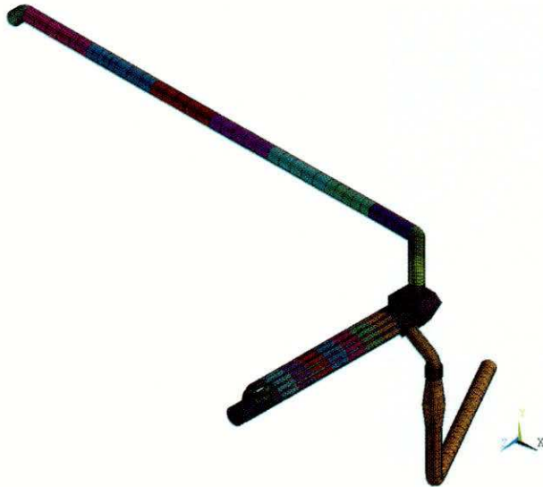
Fig. 2. Plot of ANSYS Model Showing Air Intake / Exhaust Ducting, Exhaust Plenum Chamber, Main 20" Firetubes and 6x6" Exhaust Firetubes.
