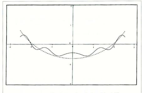
Fig. 1. Concave wall and optimised amplitude modulated diffuser
