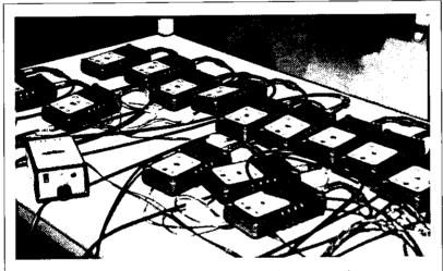
Fig. 5. CEL-460 noise dosimeters undergoing soak testing
