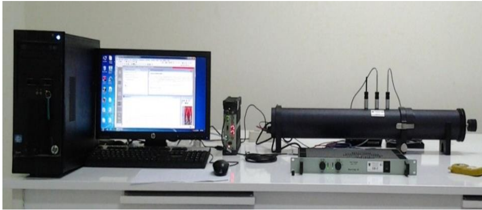
Figure 3: Absorption coefficients measurement with impedance tube
