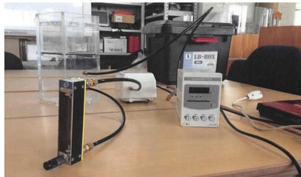
Figure 4: Flow resistivity measurement set up
