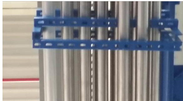
Figure 9: Clamping tube bundle and shell Isolation
