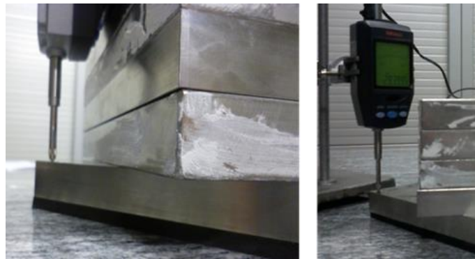
Figure 2: Measurement of thickness decreasing, as a function of static load.
