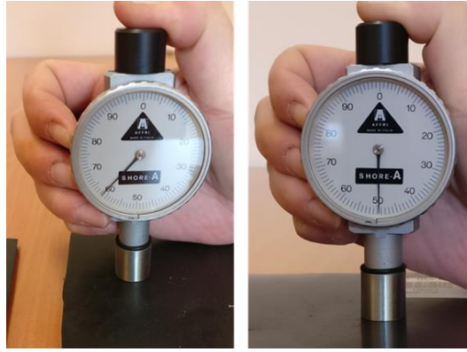
Figure 1: Measurement of shore-A hardness, by using a calibrated tester.
