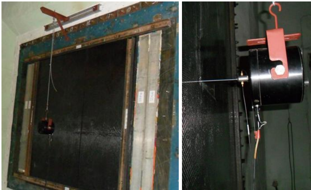
Figure 3: Vibration exciter on a suspension (view from side of RC1).
