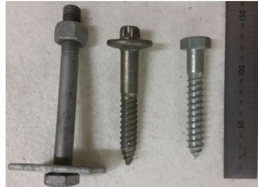
Figure 3 Shear connectors, left-to-right bolt #16, dog screw #16, coach screw #16.
