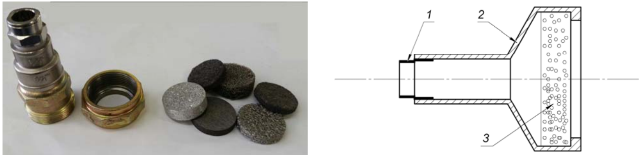
a) muffler appearance; б) muffler design diagram 1 – air supply fitting; 2 – muffler casing; 3 – porous part Figure 2 – Muffler
