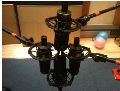
Figure 3: Blumlein-omnidirectional (Ambisonics) microphone array
