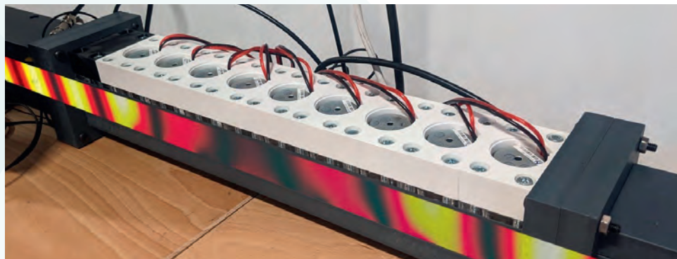
Above: Figure 2: Experimental setup for demonstrating the quantum tunnelling effect realised using the active acoustic metamaterials developed in the project. This photograph shows the rectangular duct with an array of nine loudspeakers attached to the top wall of the duct, representing the active metamaterial unit cells. The colour map along the centre of the duct is a computer-generated overlay created using a simulation model, illustrating the tunnelling of a sound wave through the metamaterial
