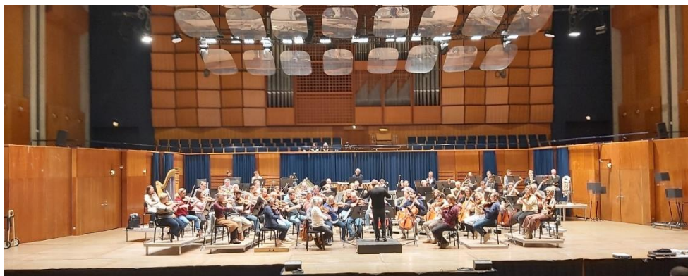
Fig. 5 The hall on November 17 th (2nd day) with more and higher risers and reduced curtain area. Two of the three plexiglass reflector arrays are also visible
