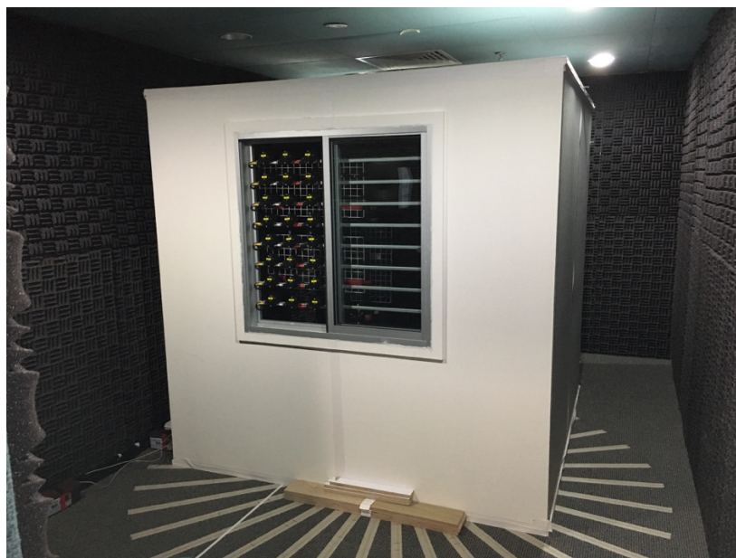
Figure 4: A full scale test chamber measuring 2 \times 2 \times 2 \text{ m}^3 , located in a recording studio. The sliding window installed on one side of the chamber measures 1 \times 1 \text{ m}^2 .
