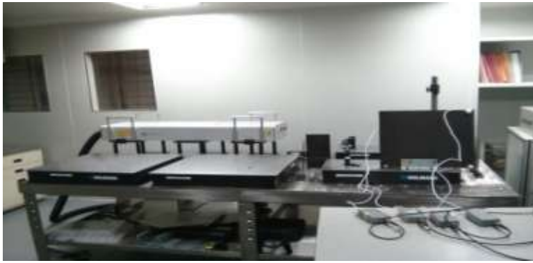
Figure 3. Experimental set up for Acoustic Wave propagation using LASER source
