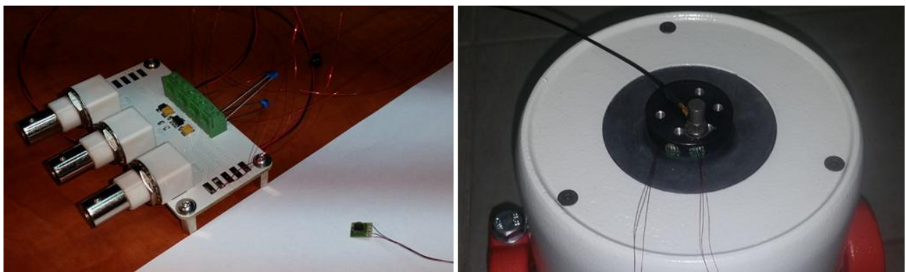
Figure 3: Left: ultralight accelerometer, power supply. Right: calibration of the accelerometers.
