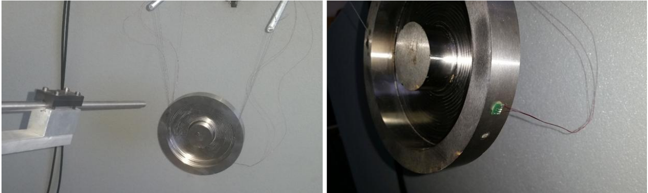
Figure 6: Left: suspended disc, automated pneumatic ball shooter. Right: Xtrinsic accelerometer attached on the side of the rim.
