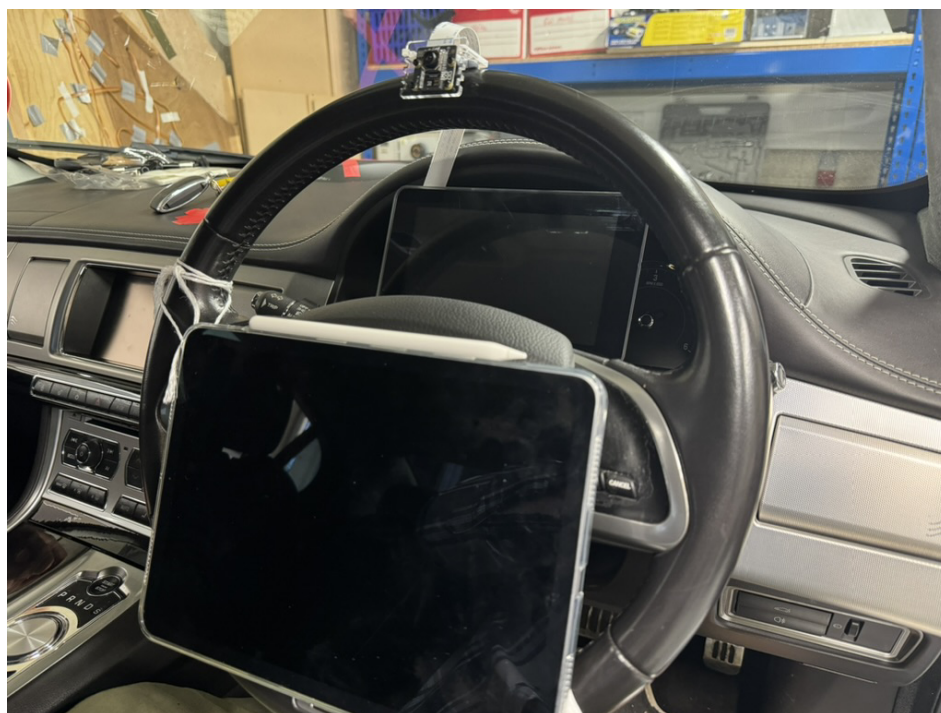
Figure 3 – iPad and webcam mounted on the steering wheel. The screen for the Raspberry Pi head tracker is fixed in front of the instrument cluster and can be seen through the steering wheel
