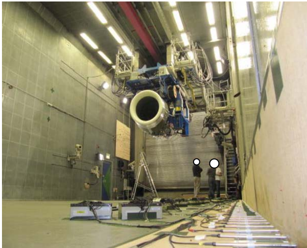
Figure 5 Dahlewitz test cell: BR700 series engine with DLR linear array (right corner)
