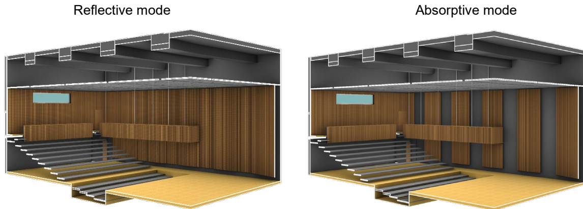
Figure 4 Acoustic models for the reflective (left) and absorptive (right) venue configurations.
