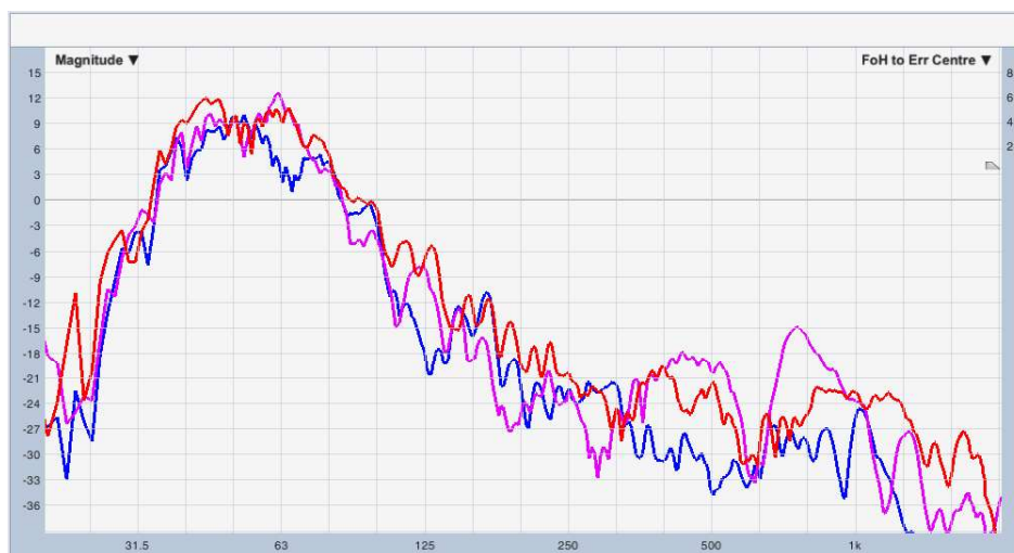
Figure 8: Smart RTA measurements at the point of immission. The transfer function of three error microphone positions (shown in figure 7) are plotted. The data is smoothed over 1/12 octave.
