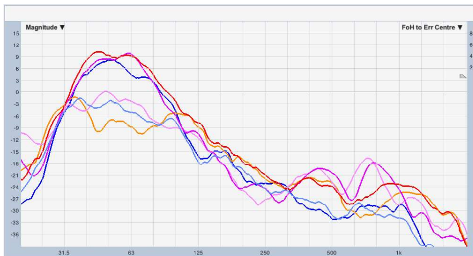
Figure 9: Efficiency of the LMS-based ANC algorithm. The bright lines show measurements while the ANC system is turned on, compared to the dark lines where the ANC System is turned off. A SPL reduction up to 18 dB is achieved around 50 Hz. The data is smoothed over 1/3 oct. The red (ANC off) and the orange (ANC on) curves belong to the central measurement position in figure 7. The other four curves belong to the lateral microphone positions.
