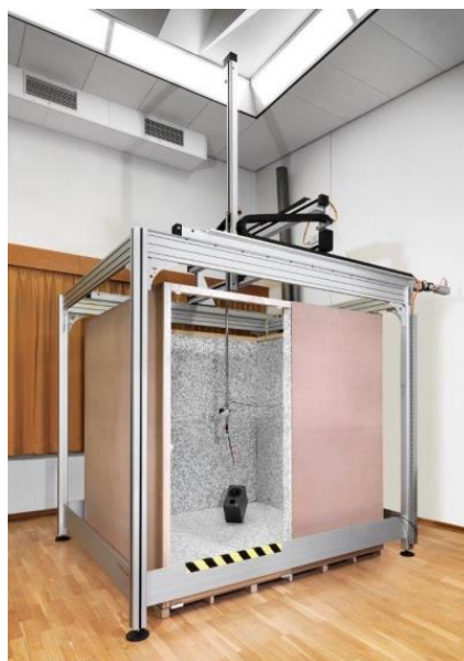
Figure 3: PTB scanning system with implemented free-field environment with a volume of approximately 2 m x 2 m x 2 m.
