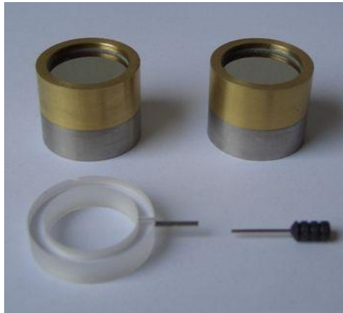
Figure 1: Two lapped LS1P-microphones B&K 4160 and a sapphire coupler with sealing needle.
