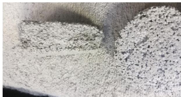
Figure 10: System B. Samples obtained from the specimen tested in the reverberant room before (background and left) and after (right) the working out of the surface.
