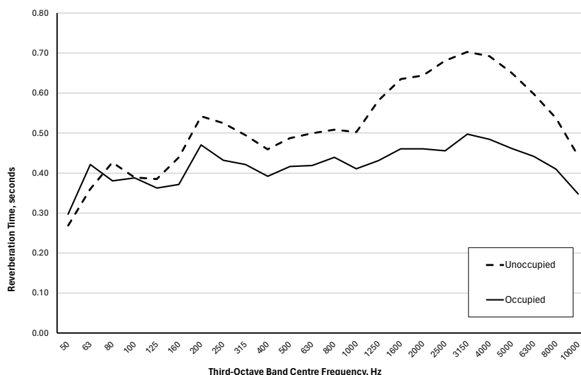
Figure 2: Reverberation Time measured without active acoustics system on (passive mode), in the occupied (approx. 70%) and unoccupied state.
