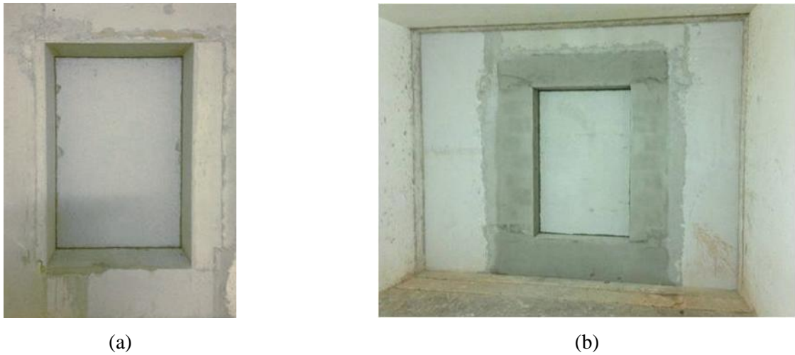
Figure 1: Installation of the plasterboard (a) and the gypsum fibreboard (b) panels in double transmission room according to ISO 10140-1, annex D.
