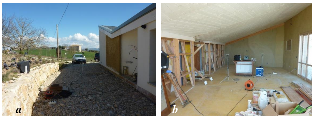
Figure 3: a) Façade sound insulation and b) reverberation time measurements.
