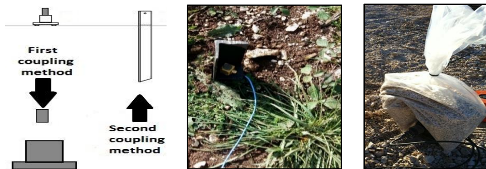
Fig. 1 : drawing of the coupling methods (left figure), positioning of transducer on the iron spike (central figure) and use of a rock sack (right figure)
