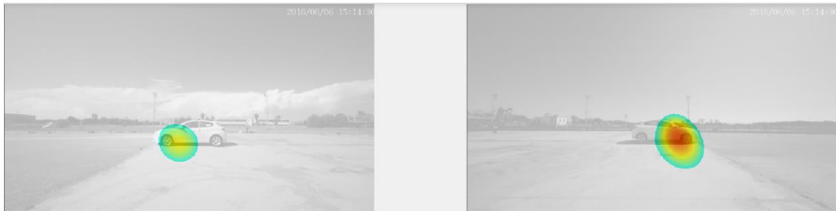
Figure 7: Pass-by-noise test with standard tyres: 20 km/h
