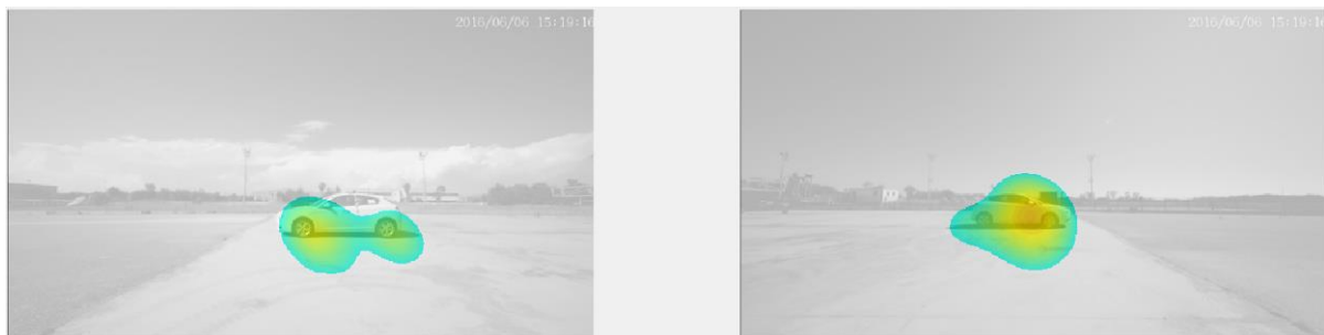
Figure 8: Pass-by-noise test with standard tyres: 30 km/h
