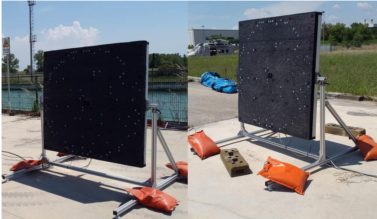
Figure 5: CIRA acoustic antennas
