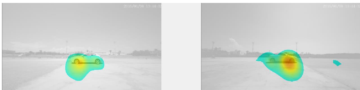
Figure 13: Pass-by-noise test with optimized tyres: 40 km/h
