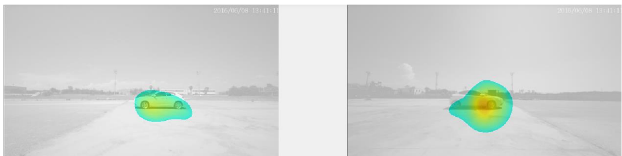
Figure 12: Pass-by-noise test with optimized tyres: 30 km/h
