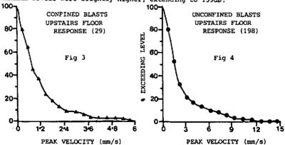
Similar distributions are shown in figures 3 and 4 where the resulting vibration response of the upstairs floor is considered. The extent of the variation demonstrates the need to monitor the effects of a number of blasts before a true picture of likely maximum vibration levels, can be determined at a particular location.
