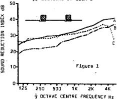
The critical frequency, the onset of coincidence resonance, for lead clad steel occurs at around 15000 Hz, well up the audio frequency range. For equivalent weight steel the figure is around 5000 Hz. Although many common sounds have predominant frequencies below the letter frequency a great deal of industrial noise extends well up the frequency range and hence the superior performance of lead clad steel can be used to advantage.
