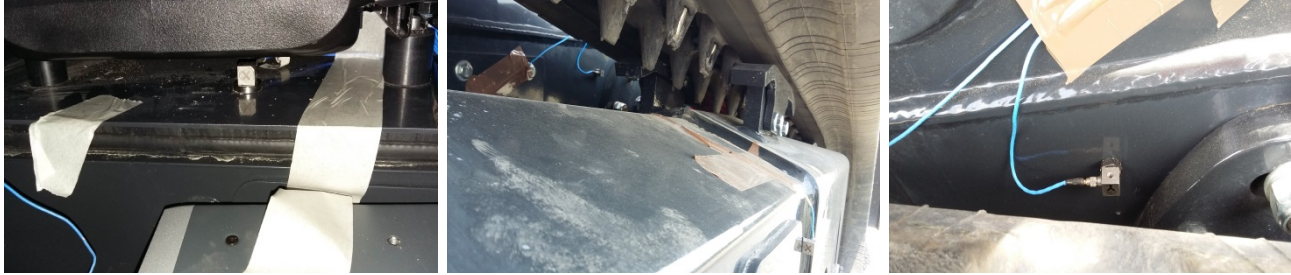
Figure 3: Structural vibration measurements at seat base (left, FLOOR), track undercarriage frame (central, T 1 ) and loader main frame (right, T 2 ).
