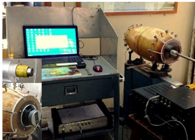
Figure 10: Experimental Setup : Wooden Shell Cavity Inset : Microphone and Speaker
