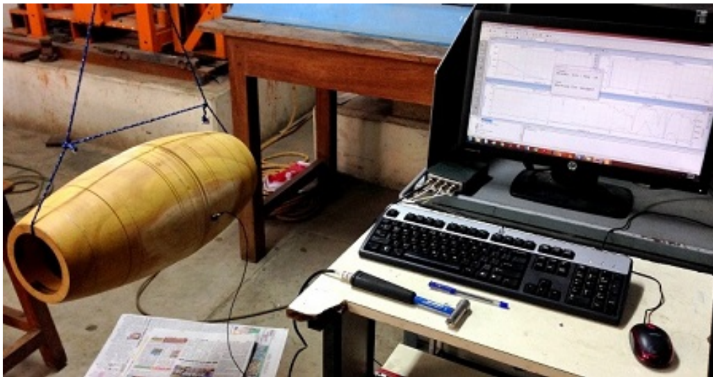
Figure 2: Experimental Setup - Mridangam Body Modal Analysis
