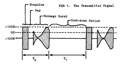
receiver decoder with the incoming signal it was considered desirable to precede each transmission with a constant-amplitude prepulse (the knowledge that this was of constant amplitude was also used at the receiver for the purposes of automatic gain control), and the transmitted signal was as shown in Fig. 1 (illustrated for the case of 100% modulation with a sine wave).
