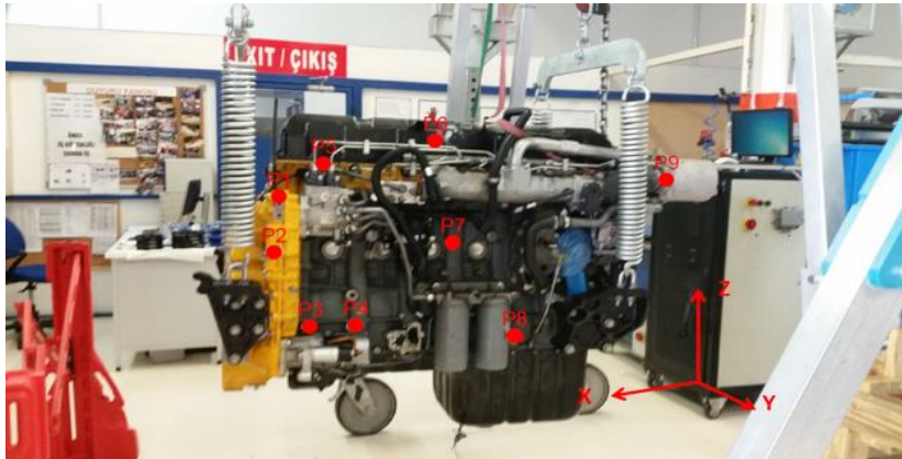
Figure 3: Engine Mass Moment of Inertia Testing
