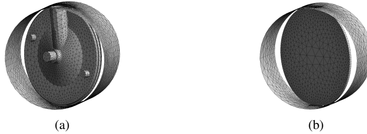
Figure 2: Surface discretization around the butterfly valve for (a) the detailed geometry and (b) the simplified geometry.
