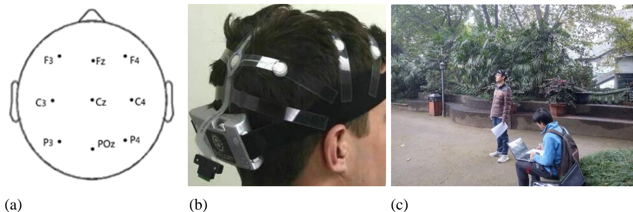
Figure 2. EEG electrode placement (a) Electrode position schematically, considering Fz, F3, F4, Cz, C3, C4, POz, P3, and P4 regions (b) Electrode installation instructions, (c) Field experiment.
