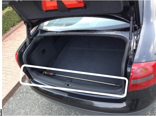
Fig.1 Performance damper installed on a car
