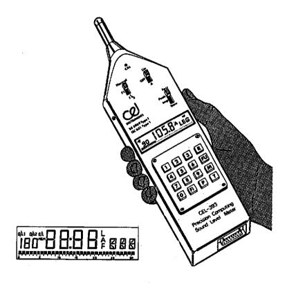
Fig.1. CEL-393 Precision Computing Sound Level Meter with inset showing display.
