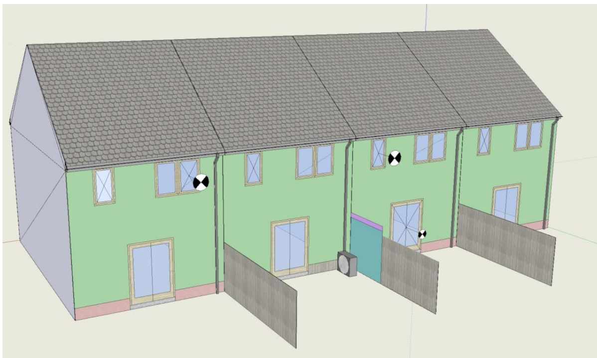
Figure 7: illustration of the ASHP unit arranged with its back to the fence, with a taller barrier portion (here shown at 2.0 m), extending 2 m from the house only, with the remaining fence shown at 1.8
