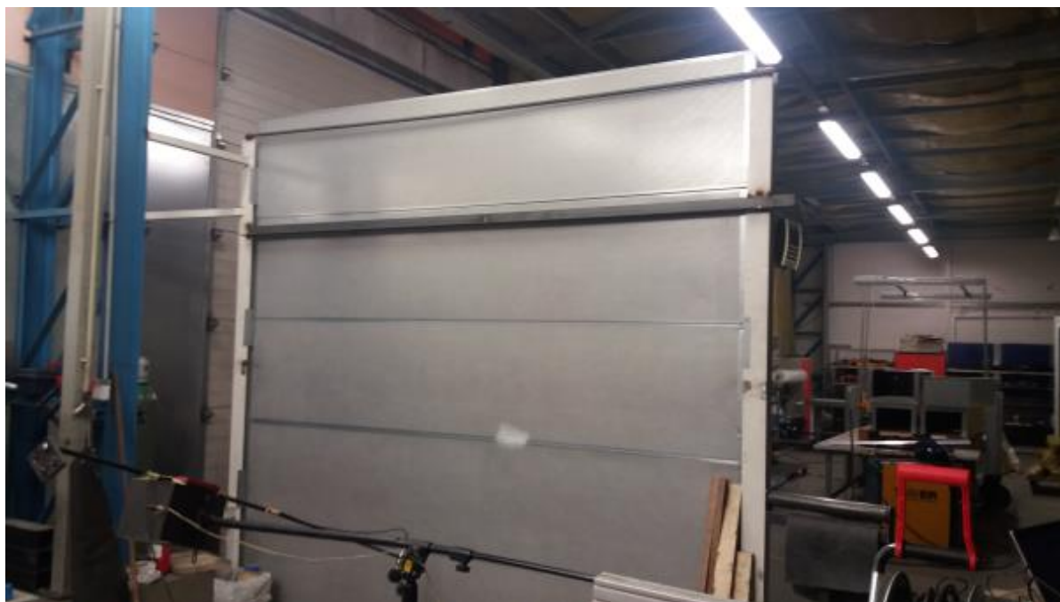
Figure 5: Photo of prototype noise barrier made of acoustic panels by KFB
