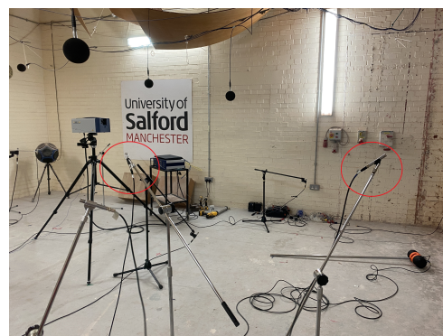
(b) Photograph of microphone arrangement inside the room under test, with the microphones used circled in red.
