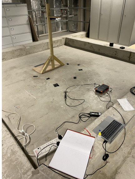
(a) Test setup on the primary structure
