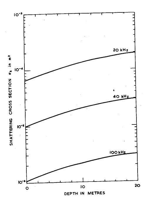
FIG. I. VARIATION OF SCATTERING CROSS-SECTION WITH DEPTH
