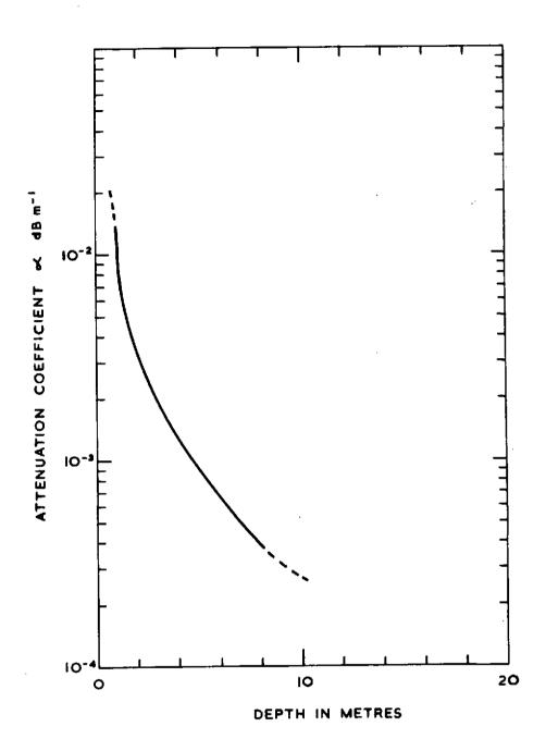
FIG. 5. ATTENUATION PROFILE FOR RESULTS OF FIG. 4. (SEA STATE I)
