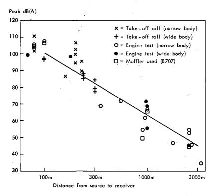
Fig. 1 Relationship between take-off roll and engine test noise and distance from the source.
