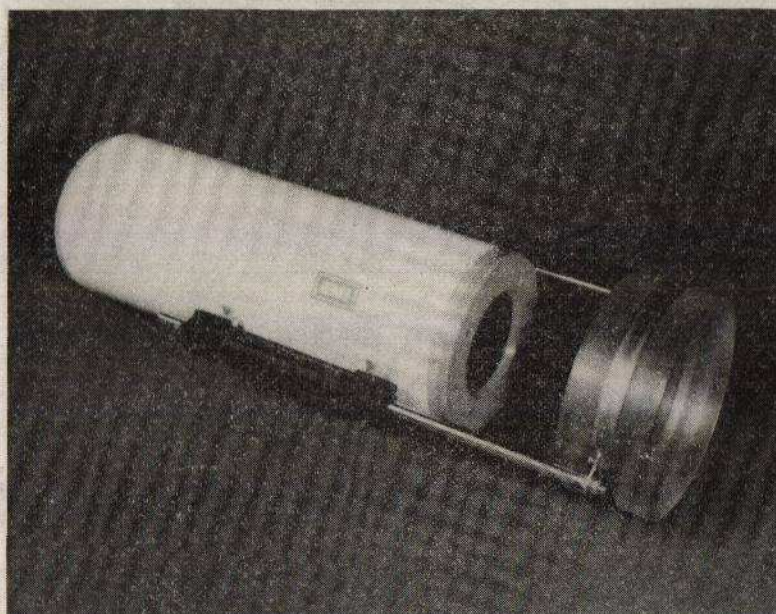
ULTRASONIC CAMERA FOR IMMERSION TO 300 METRES DEPTH
